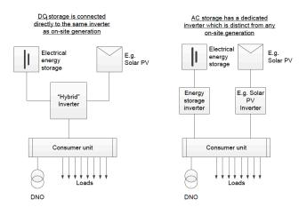
Figure 1: DC- and AC-connected energy storage
